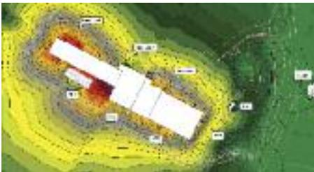
**Odour and litter:** Waste will be handled within a fully enclosed building to prevent the release of odour and litter from the facility. In addition air will be extracted from the waste tipping hall as part of the combustion process. This will result in a slight negative air pressure that prevents odour and litter from escaping the building.
